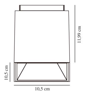
Voltage (V): 230 Volt IP degree: IP20 Maximum bulb wattage (W): 50 Class (Class 1, Class 2, Class 3): Class 2 (Double isolated) Socket type: GU10 Parallel connection: True
