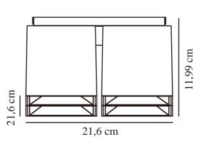
Voltage (V): 230 Volt IP degree: IP20 Maximum bulb wattage (W): 4x50W
