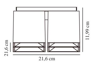
Voltage (V): 230 Volt IP degree: IP20 Maximum bulb wattage (W): 50 Class (Class 1, Class 2, Class 3): Class 2 (Double isolated) Socket type: GU10 Parallel connection: True
