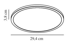
Voltage (V): 230 Volt IP degree: IP54 Class (Class 1, Class 2, Class 3): Class 2 (Double isolated) Socket type: LED - Nonreplaceable light source Dimmerable: False
