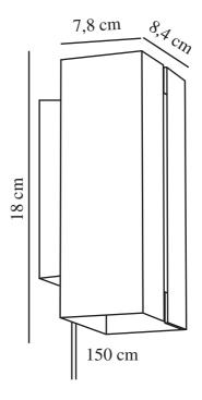
Voltage (V): 230 Volt IP degree: IP20 Class (Class 1, Class 2, Class 3): Class 2 (Double isolated) Socket type: LED Module Dimmerable: True
