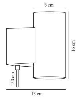
Voltage (V): 230 Volt IP degree: IP20 Class (Class 1, Class 2, Class 3): Class 2 (Double isolated) Socket type: LED Module Switch placement: On the cable Parallel connection: False
