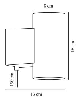
Voltage (V): 230 Volt IP degree: IP20 Class (Class 1, Class 2, Class 3): Class 2 (Double isolated) Socket type: LED Module Switch placement: On the cable Parallel connection: False
