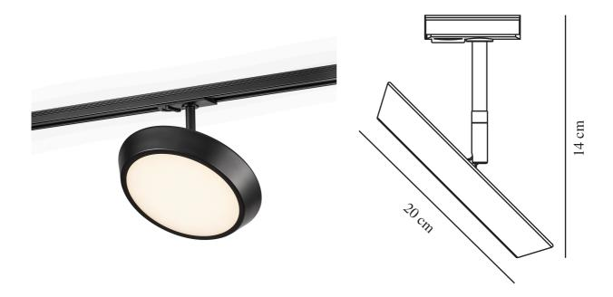
Voltage (V): 230 Volt IP degree: IP20 Class (Class 1, Class 2, Class 3): Class 1 (Earth contact) Socket type: LED Module Dimmerable: True
