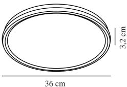
Voltage (V): 220-240 Volt IP degree: IP54 Class (Class 1, Class 2, Class 3): Class 2 (Double isolated) Socket type: LED Module Parallel connection: False
