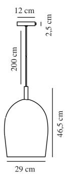
Voltage (V): 230 Volt IP degree: IP20 Maximum bulb wattage (W): 40W Class (Class 1, Class 2, Class 3): Class 1 (Earth contact) Socket type: E27
