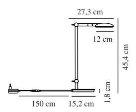
Voltage (V): 230 Volt IP degree: IP20 Class (Class 1, Class 2, Class 3): Class 3 (12V) Socket type: LED Module Switch placement: On the fixture
