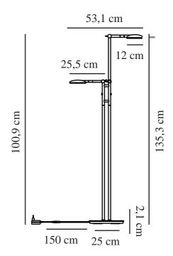
Voltage (V): 230 Volt IP degree: IP20 Class (Class 1, Class 2, Class 3): Class 3 (12V) Socket type: LED Module Switch placement: On the fixture
