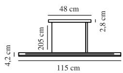
Voltage (V): 230 Volt IP degree: IP20 Class (Class 1, Class 2, Class 3): Class 2 (Double isolated) Socket type: LED – Nonreplaceable light source
