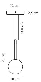
Voltage (V): 230 Volt IP degree: IP20 Maximum bulb wattage (W): 5 Class (Class 1, Class 2, Class 3): Class 2 (Double isolated) Socket type: G9
