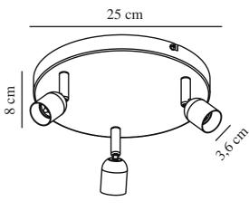
Voltage (V): 220-240 Volt IP degree: IP20
