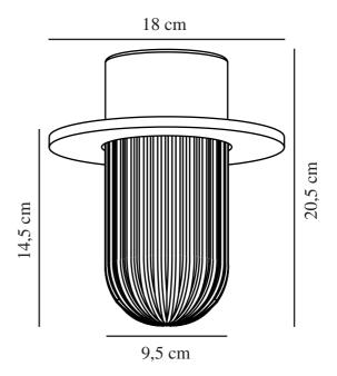
Voltage (V): 220-240 Volt IP degree: IP54 Maximum bulb wattage (W): 60W Class (Class 1, Class 2, Class 3): Class 2 (Double isolated) Socket type: E27
