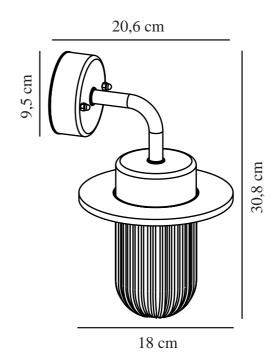
Voltage (V): 220-240 Volt IP degree: IP54
