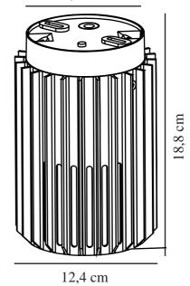
Voltage (V): 220-240 Volt IP degree: IP54 Maximum bulb wattage (W): 15 Class (Class 1, Class 2, Class 3): Class 1 (Earth contact) Socket type: E27 Parallel connection: True
