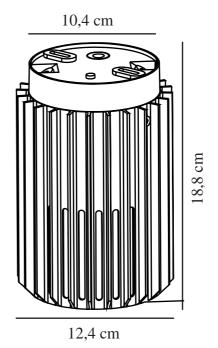
Voltage (V): 220-240 Volt IP degree: IP54 Maximum bulb wattage (W): 15W Class (Class 1, Class 2, Class 3): Class 1 (Earth contact) Socket type: E27
