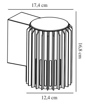
Voltage (V): 220-240 Volt IP degree: IP54 Maximum bulb wattage (W): 15
