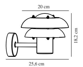
Voltage (V): 230 Volt IP degree: IP54 Maximum bulb wattage (W): 12W Class (Class 1, Class 2, Class 3): Class 1 (Earth contact) Socket type: E14 Parallel connection: True
