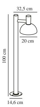
Voltage (V): 230 Volt IP degree: IP54 Maximum bulb wattage (W): 20 Class (Class 1, Class 2, Class 3): Class 1 (Earth contact) Socket type: E27 Parallel connection: True
