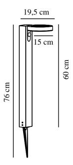
IP degree: IP44 Class (Class 1, Class 2, Class 3): Class 3 (12V) Socket type: SolarLed
