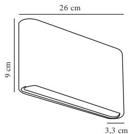
Voltage (V): 230 Volt IP degree: IP54 Class (Class 1, Class 2, Class 3): Class 1 (Earth contact) Socket type: LED – Nonreplaceable light source Parallel connection: True
