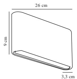
Voltage (V): 230 Volt IP degree: IP54 Class (Class 1, Class 2, Class 3): Class 1 (Earth contact) Socket type: LED – Nonreplaceable light source Parallel connection: True
