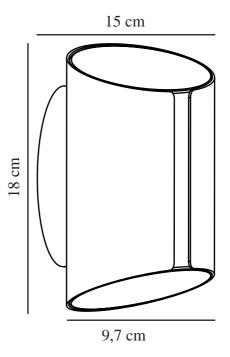
Voltage (V): 220-240 Volt IP degree: IP54
