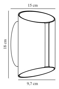
Voltage (V): 220-240 Volt IP degree: IP54 Class (Class 1, Class 2, Class 3): Class 1 (Earth contact) Socket type: LED - Nonreplaceable light source Parallel connection: True
