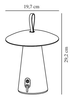
IP degree: IP54 Class (Class 1, Class 2, Class 3): Class 3 (12V) Socket type: LED Module Switch placement: On the base
