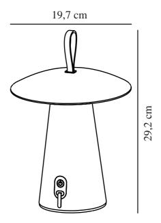
IP degree: IP54 Class (Class 1, Class 2, Class 3): Class 3 (12V)
