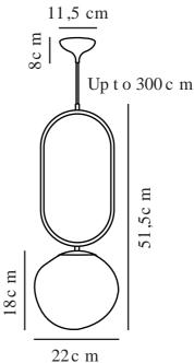
Voltage (V): 230 Volt IP degree: IP20 Maximum bulb wattage (W): 15W Class (Class 1, Class 2, Class 3): Class 2 (Double isolated) Socket type: E27
