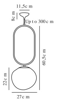
Voltage (V): 230 Volt IP degree: IP20 Maximum bulb wattage (W): 15 Class (Class 1, Class 2, Class 3): Class 2 (Double isolated) Socket type: E27
