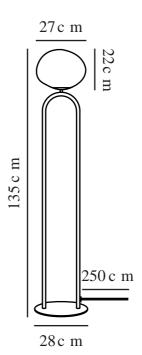
IP degree: IP20 Maximum bulb wattage (W): 15 Class (Class 1, Class 2, Class 3): Class 2 (Double isolated) Socket type: E27
