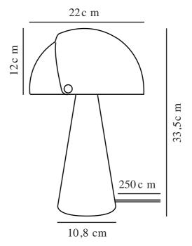
Voltage (V): 230 Volt IP degree: IP20 Maximum bulb wattage (W): 25 Class (Class 1, Class 2, Class 3): Class 2 (Double isolated) Socket type: E27 Switch placement: On the cable
