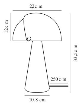
Voltage (V): 220-240 Volt IP degree: IP20 Maximum bulb wattage (W): 25 Class (Class 1, Class 2, Class 3): Class 2 (Double isolated) Socket type: E27
