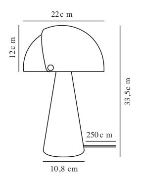
Voltage (V): 220-240 Volt IP degree: IP20 Maximum bulb wattage (W): 25 Class (Class 1, Class 2, Class 3): Class 2 (Double isolated) Socket type: E27 Switch placement: On the cable
