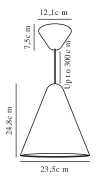
Voltage (V): 220-240 Volt IP degree: IP20 Maximum bulb wattage (W): 40W Class (Class 1, Class 2, Class 3): Class 2 (Double isolated) Socket type: E27
