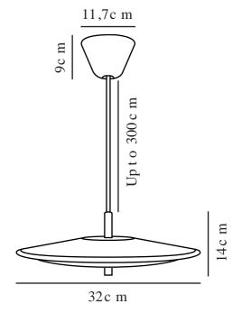
Voltage (V): 230 Volt IP degree: IP20 Class (Class 1, Class 2, Class 3): Class 2 (Double isolated) Socket type: LED Module Dimmerable: True
