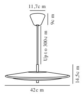
Voltage (V): 230 Volt IP degree: IP20 Class (Class 1, Class 2, Class 3): Class 2 (Double isolated) Socket type: LED Module
