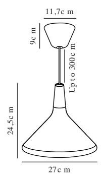
Voltage (V): 230 Volt IP degree: IP20 Maximum bulb wattage (W): 40W Class (Class 1, Class 2, Class 3): Class 2 (Double isolated) Socket type: E27
