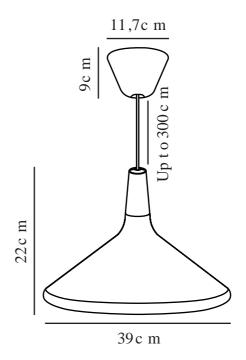
Voltage (V): 230 Volt IP degree: IP20 Maximum bulb wattage (W): 40 Class (Class 1, Class 2, Class 3): Class 2 (Double isolated) Socket type: E27
