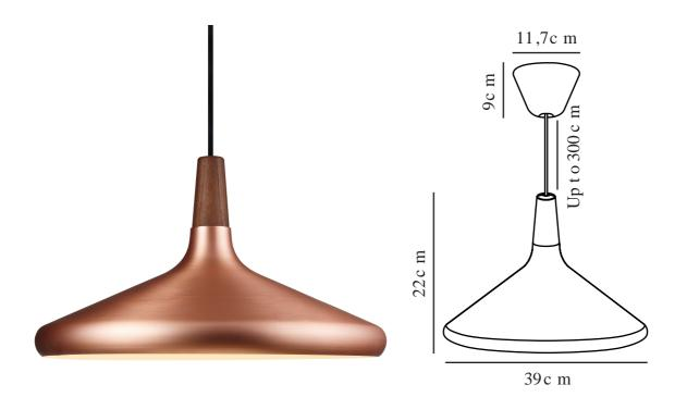
Voltage (V): 230 Volt IP degree: IP20 Maximum bulb wattage (W): 60W Class (Class 1, Class 2, Class 3): Class 2 (Double isolated) Socket type: E27 Dimmerable: Yes with compatible bulb
