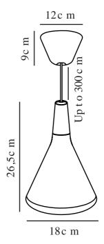
Voltage (V): 230 Volt IP degree: IP20
