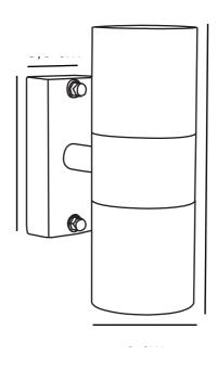
Voltage (V): 230 Volt IP degree: IP54 Maximum bulb wattage (W): 35 Class (Class 1, Class 2, Class 3): Class 1 (Earth contact) Socket type: GU10 Parallel connection: False
