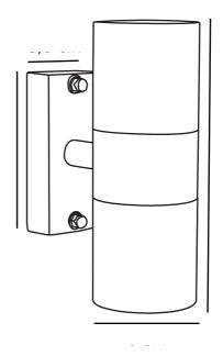
Voltage (V): 230 Volt IP degree: IP54 Maximum bulb wattage (W): 2X35W
