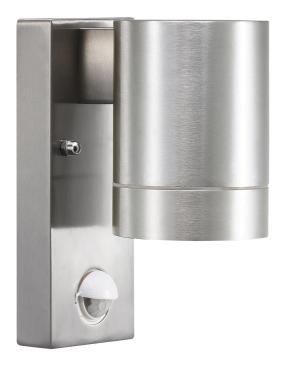
Voltage (V): 230 Volt IP degree: IP54 Maximum bulb wattage (W): 35W Class (Class 1, Class 2, Class 3): Class 1 (Earth contact) Socket type: GU10 Parallel connection: True
