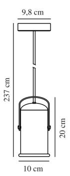
Voltage (V): 220-240 Volt IP degree: IP20 Maximum bulb wattage (W)
