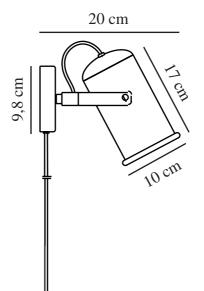
Voltage (V): 220-240 Volt IP degree: IP20 Maximum bulb wattage (W): 60W Class (Class 1, Class 2, Class 3): Class 2 (Double isolated) Socket type: E27 Switch placement: On the cable Parallel connection: True
