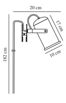
Voltage (V): 220-240 Volt IP degree: IP20
