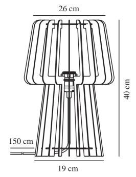
IP degree: IP20 Maximum bulb wattage (W): 40W Class (Class 1, Class 2, Class 3): Class 2 (Double isolated) Socket type: E27
