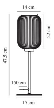
Voltage (V): 220-240 Volt IP degree: IP20
