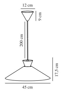
Voltage (V): 220-240 Volt IP degree: IP20
